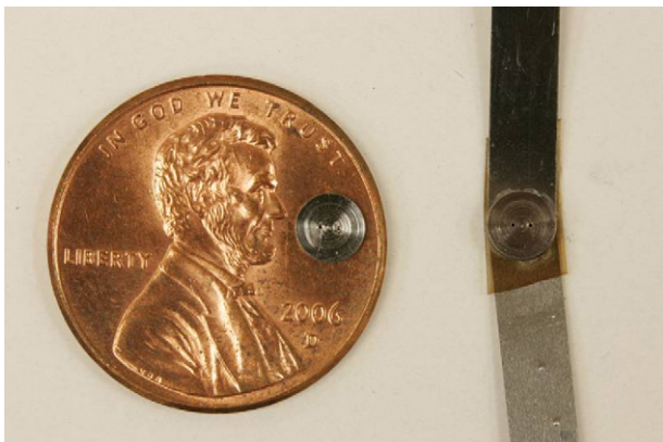
Fig. 2. 11 mm 3 cell placed on top of a penny (left) and another cell of same design with extended stainless steel plates for electrical connection (right).
